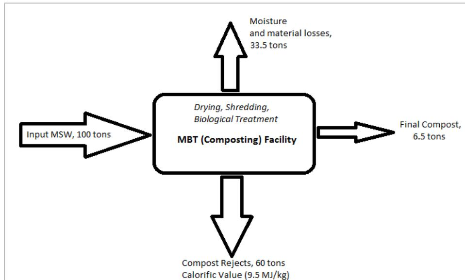
Figure 28, Material Balance Flowchart of MBT Process, with Calorific Values of Different Fractions of Composting Rejects: Source: Ramky Enviro Engineers
