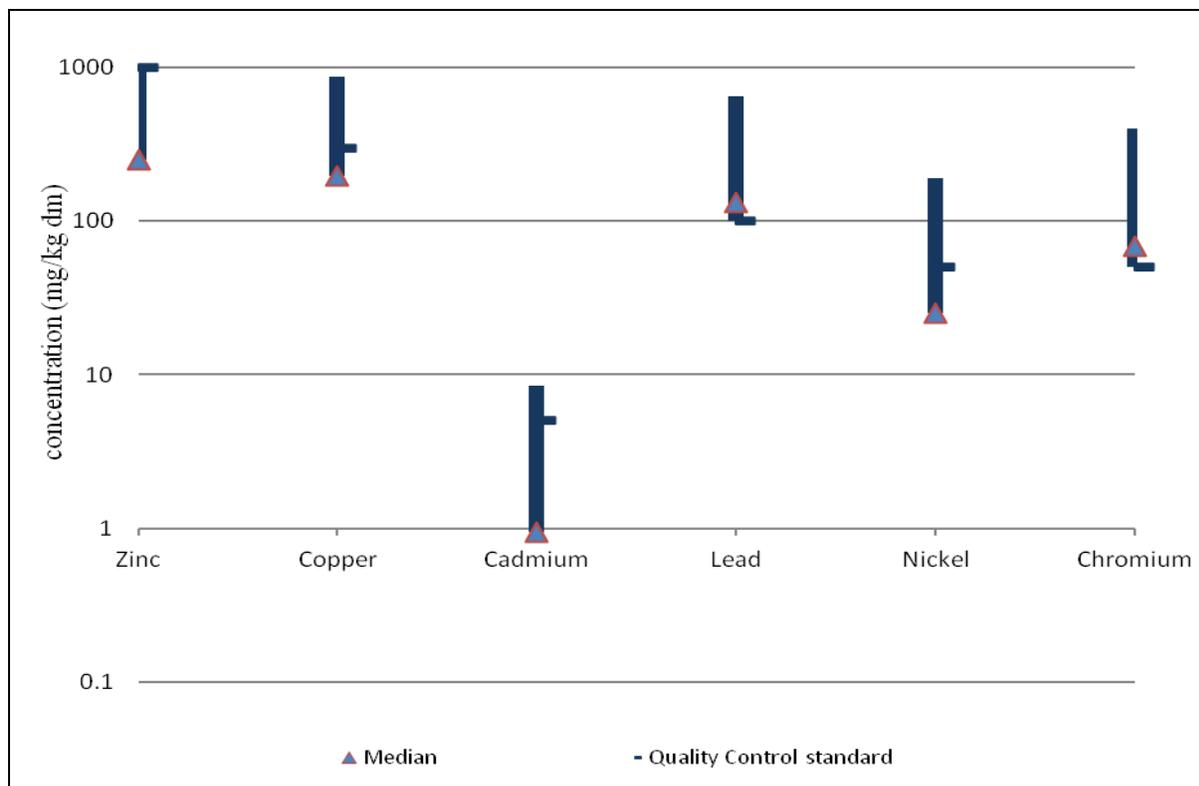
**Figure 29, Heavy Metals Concentration in Mixed Solid Waste Compost in Comparison to Quality Control Standards**
