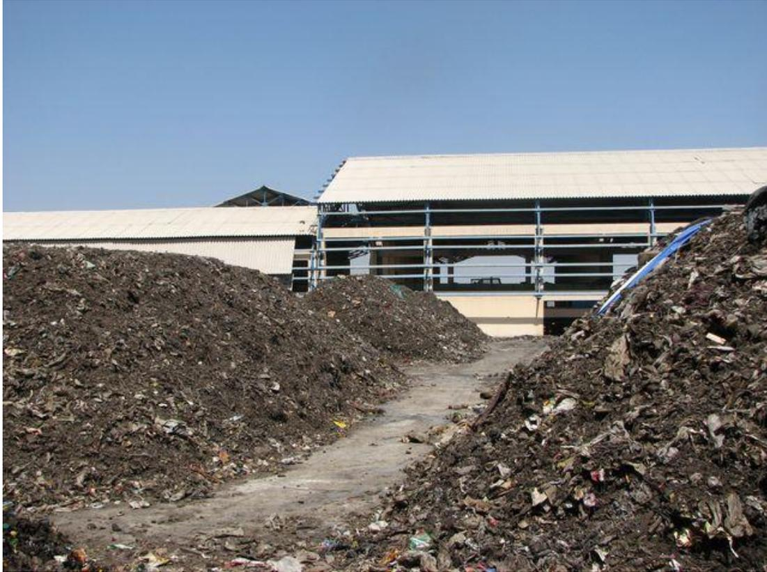
Figure 27, Windrow Composting of mixed solid wastes is the most successful waste management technology in India
