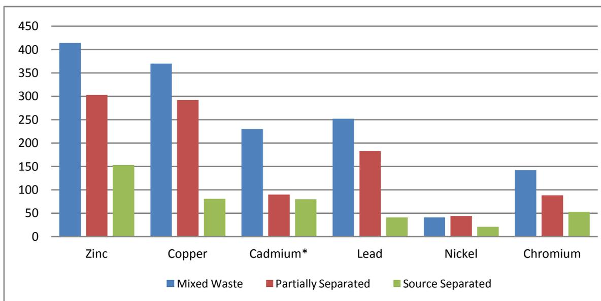
**Figure 38, Impact of Source Separation on Heavy Metals Concentration in MSW Compost**
