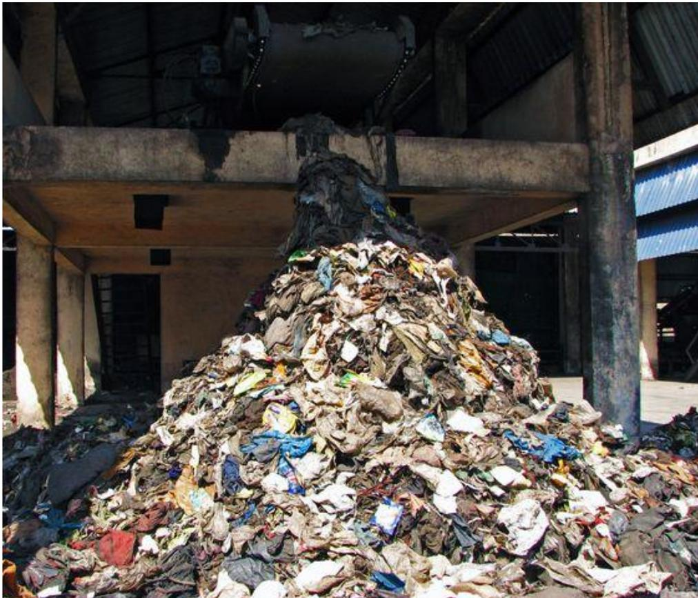
**Figure 32, Composting Rejects are up to 60% of Input MSW and have a Calorific Value as high as 11.6 MJ/kg**
