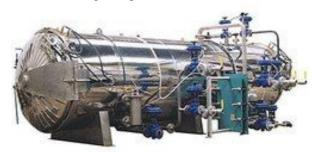
Fig 5 Autoclave
