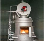
Fig 4 Incinerator for contraband drugs
